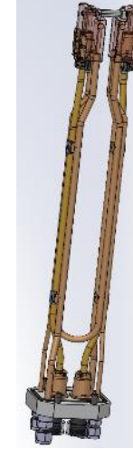
Internal source for small cyclotrons
